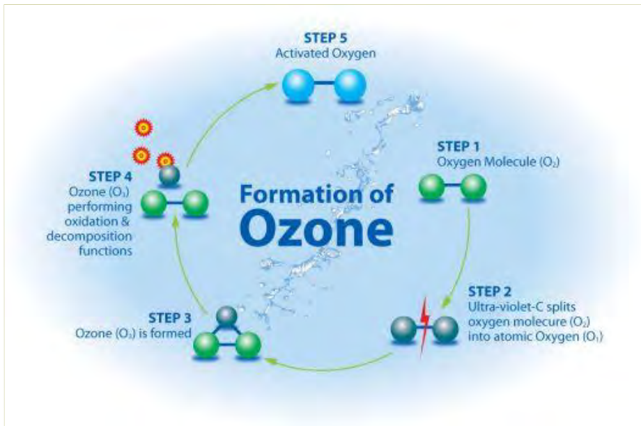
Figure 4: Ozone process diagram
